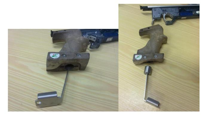
2. Detach the grip holding bolt by pressing the pin, and change it to the longer bolt for wooden grip
