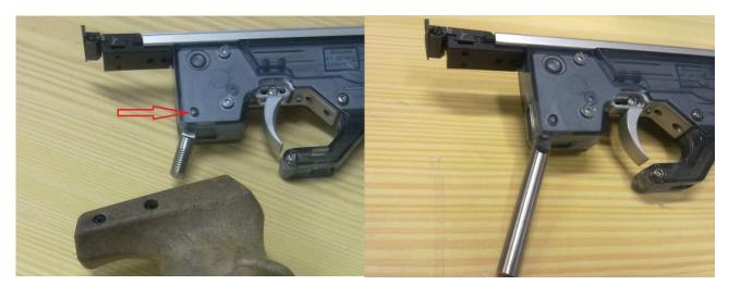
3. Attach the wooden grip to its place, and tighten it with 4mm allen key.
